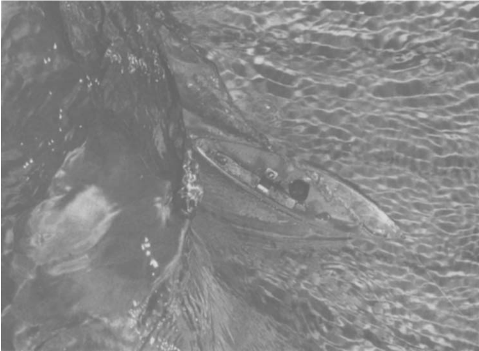
FIGURE 14. Top view of transparent surfboard model riding the wave. The cross marks the centre-of-mass position. Note the leading edge of the wetted area and the starboard side capillary waves.
