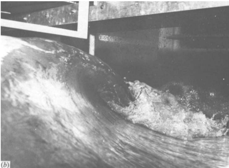
FIGURE 4. (a) Desirable wave shape showing a surfer in a somewhat bumpy ride. (b) Model wave produced in the flume.
